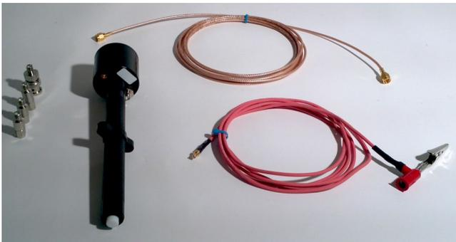
The CDMES uses an enclosed mechanical gap control system to simulate the electrostatic discharge which occurs between a charged object and a ground reference. Specifically, it simulates the Charged Device Model (CDM) discharge type which is characterized by a fast single-peak pulse waveform of transferred current between the device and ground.
