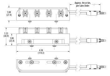
Note: The use of the air-assist kit feature will change the thickness from 1.08'' (27.4 mm) to 1.46'' (37.1 mm).
