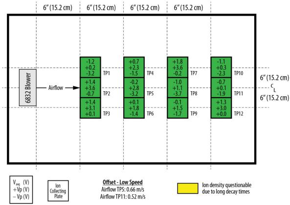
Figure 5. Offset Voltage Data - Low Speed
