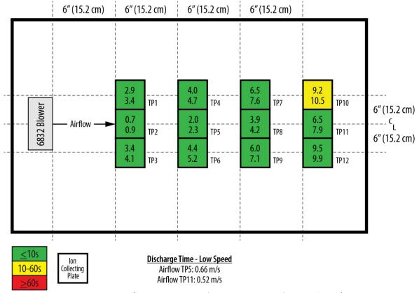
Figure 1. Discharge Time Data (±1000V to ±100V) – Low Speed
