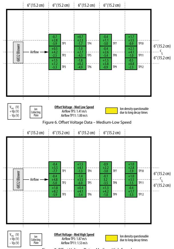
Figure 7. Offset Voltage Data – Medium-High Speed
