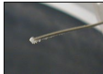
White fuzz on the tip of a tungsten wire emitter point
