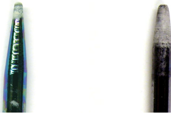
Discoloration and whitened tips on silicon (right) and titanium emitter points (left)
