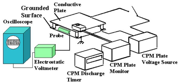
Refer to the following diagram of a possible test setup. Note that the Probe should be mounted at least 3 cm from the edge of the plate for best accuracy.
