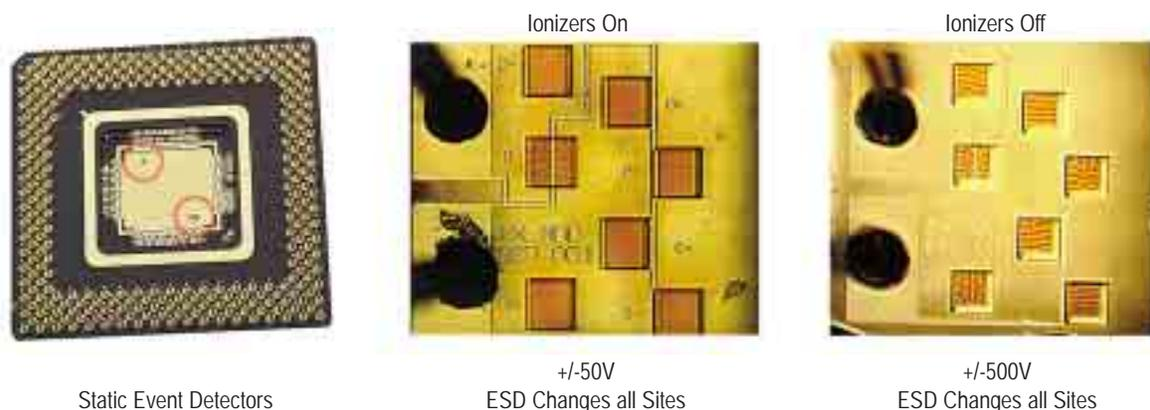
Figure 7. Static Event Detector (ExMOD)
