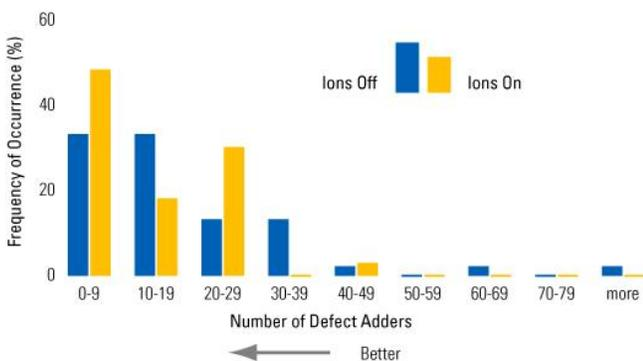
Figure 5. Etch A tool results showing the number of particles before ionization and after ionization
