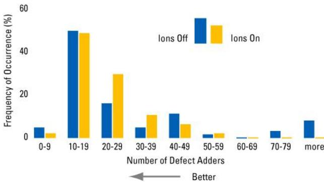
Figure 4. PVD tool results showing the number of particles before ionization and after ionization
