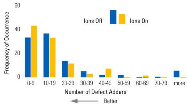
Figure 6. Etch B tool results showing the number of particles before ionization and after ionization
