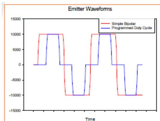
Figure 3. High and Low Duty Cycles
