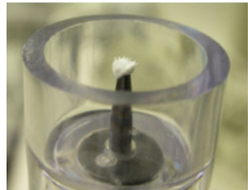
Figure 1. A White “Fuzzball” Appears On Emitter Tips As A Result Of Precipitated Materials
