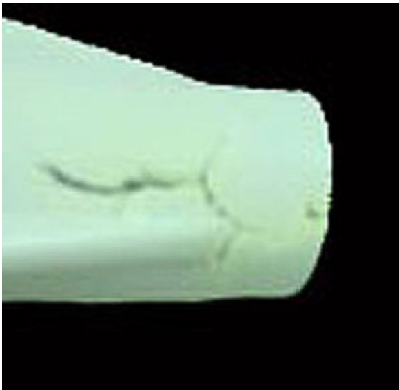
Figure 6. Cracked Nozzle From Corona
