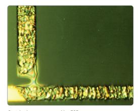
Reticle damage caused by ESD
