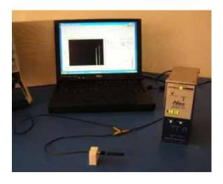
Another source of interference which has troubled ESD sensors has been the rise in general RF usage in manufacturing facilities. It is now becoming common for cell phones and two-way pagers to be authorized for use on the process floor. WiFi and Bluetooth applications are migrating into sensitive process and tool areas with the potential for disruption in ESD monitoring for very sensitive applications. RFID applications are also beginning to become popular as
