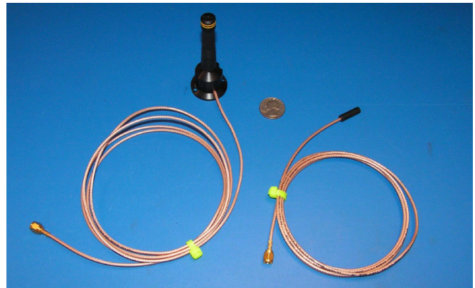
FH916 monopole antenna (standard), left; MicroESD proximity monopole antenna, right; standard Linx FH916 antenna is 6.35 cm tall, not including the base (overall height is 10.16 cm) and MicroESD antenna is 2 cm x 0.5 cm
