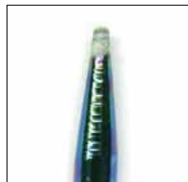
Discoloration and whitened tips on silicon (right) and titanium emitter points (left).
