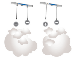
Pulsed DC systems create clouds of positive and negative ions
