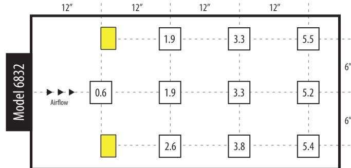
Discharge time in seconds (1000-100V), fan speed set to high; blower 12" from CPM measuring plate; CPM test plate 7.2" from table; discharge times slightly longer for 230 VAC, 50 Hz unit. Yellow cell without value = decay time over 30 seconds.
