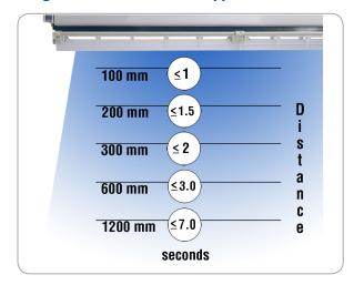
$\mu$ Wire AeroBar Model 5711 (250 mm length) with 25 mm Air Jet Spacing. Measured using Simco-lon CPM Model 280A with CDA flow at 2 l/m per air jet (18 l/m total) and no HEPA flow.
