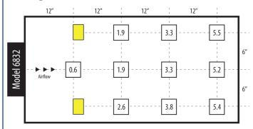
Discharge time in seconds (1000-100V), **fan speed set to high**; blower 12" from CPM measuring plate; CPM test plate 7.2" from table; discharge times slightly longer for 230 VAC, 50 Hz unit. Yellow cell without yalue = decay time over 30 seconds.
