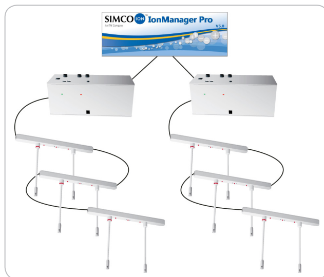
Emitters are connected to the Model 5582 Controllers, which communicate with IonManager Pro to send email notifications to a facility monitoring system or agent.
