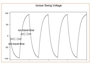
Figure 1. Ionizers using pulsed technology.
