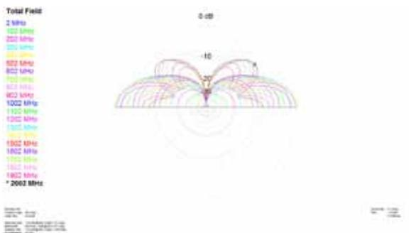
FH916 monopole antenna showing frequency range gain (on ground plane)
