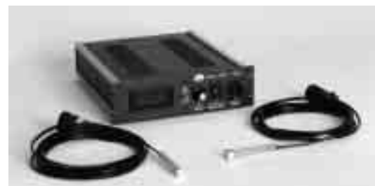
Figure 6. Indirect Charge Measurement Methods (Fieldmeter, Static Sensor, Voltmeter with Probes)
