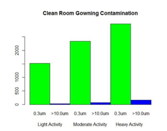
[Equipment was Lighthouse Solair 3100 with isokinetic sampling probe on tripod 6ft above floor level. Sampling was three (3) sets of three (3) each 60 second sampling intervals. Locations were just inside fab entrance door and gowning room entrance door.]
