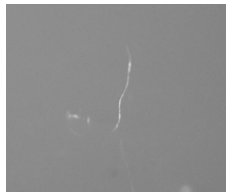
1 mm fiber standing vertically on a charged surface
