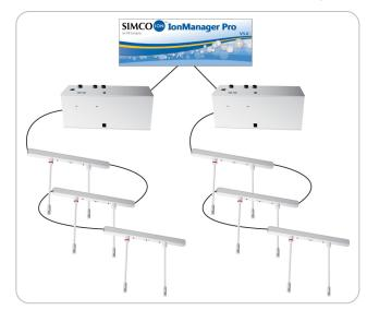
Emitters are connected to the Model 5582 Controllers, which communicate with lonManager Pro to send email notifications to a facility monitoring system or agent.
