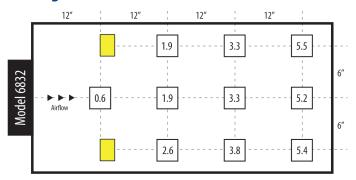
Discharge time in seconds (1000-100V), fan speed set to high; blower 12" from CPM measuring plate; CPM test plate 7.2" from table; discharge times slightly longer for 230 VAC, 50 Hz unit. Yellow cell without value = decay time over 30 seconds.
