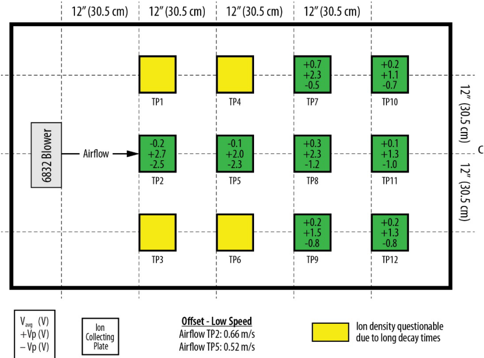
Figure 5. Offset Voltage Data – Low Speed
