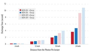
Tested by centering CPM below the ionizer. HEPA ON is with 100 fpm laminar airflow from 9.5 inch (241 mm) above the ionizer.
