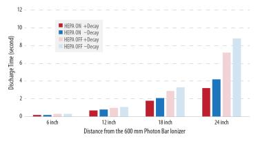
Tested by centering CPM below the ionizer. HEPA ON is with 100 fpm laminar airflow above the ionizer.
