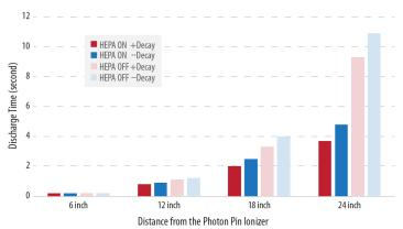
Tested by centering CPM below the ionizer. HEPA ON is with 100 fpm laminar airflow from 9.5 inch (241 mm) above the ionizer.
