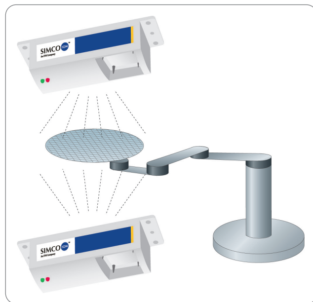
QuadBar ionizers placed above and below the wafer accelerate discharge times on the front and back surfaces, regardless of airflow.
