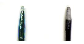
Discoloration and whitened tips on silicon (right) and titanium emitter points (left)
