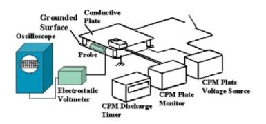
Refer to the following diagram of a possible test setup. Note that the Probe should be mounted at least 3 cm from the edge of the plate for best accuracy.
