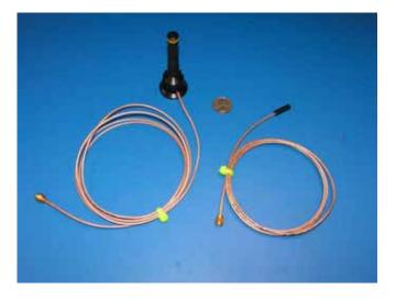
*FH916 monopole antenna (standard) is on the left; the MicroESD proximity monopole antenna is on the right, standard Linx FH916 antenna is 6.35 cm tall, not including the base (overall height is 10.16 cm) and MicroESD antenna is 2 cm x 0.5 cm*
