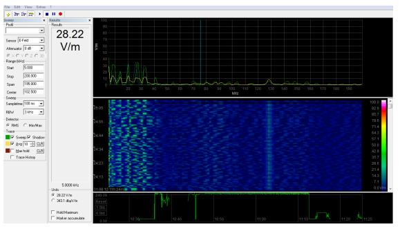
Simco-Ion 5710  $\mu Wire$  Ionizing Bar at 5" Distance from Antenna
