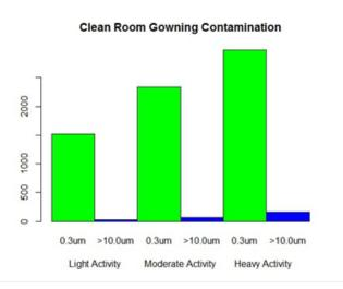
[Equipment was Lighthouse Solair 3100 with isokinetic sampling probe on tripod 6ft above floor level. Sampling was three (3) sets of three (3) each 60 second sampling intervals. Locations were just inside fab entrance door and gowning room entrance door.]
