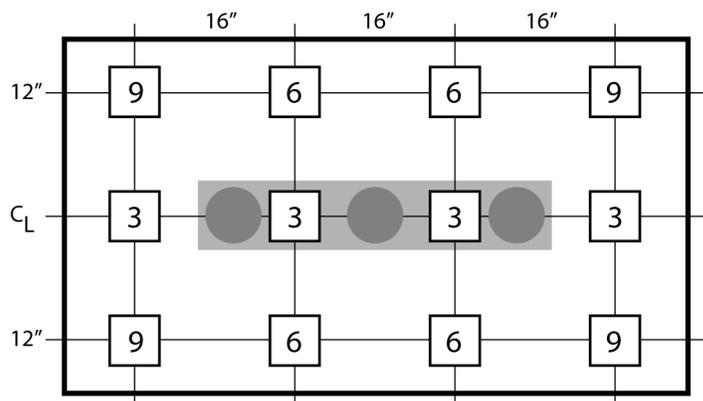
CPM test plate 6" from table; discharge times slightly longer for 230 VAC, 50 Hz unit.
